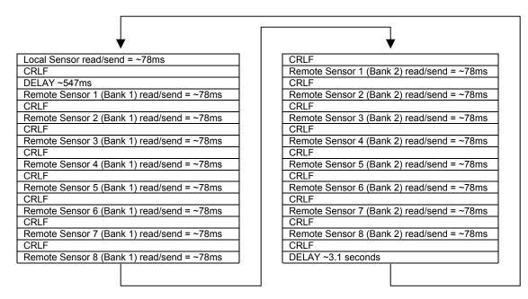
This timing applies whether additional sensors are connected or not (i.e. the single local sensor with no remote sensors attached will take about 78ms to read and transmit and will not be read and transmitted again for approximately 4.92 seconds).
